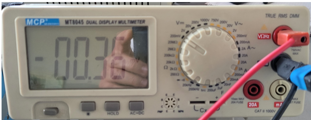
Figure 25.5. Multimeter MT8045 for measurement U_2 and calculate the photocurrent I_{photo} = U_2/10M\Omega .
