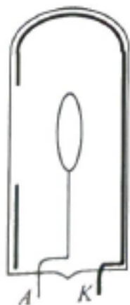
Figure 25.2. Construction of the photocell; A - anode, K - cathode
