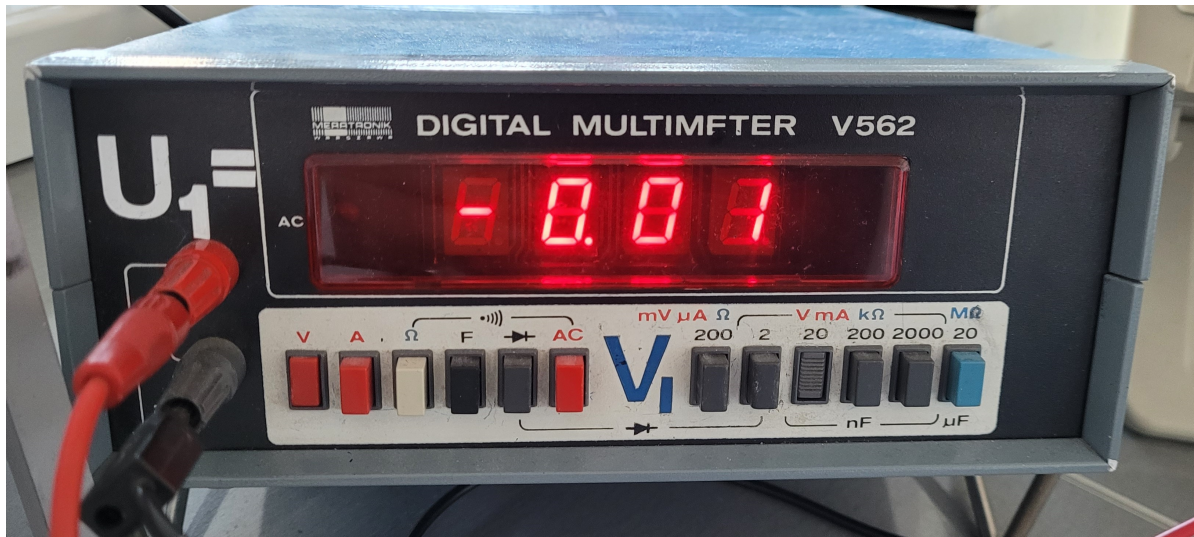
Figure 25.4. Multimeter V562 for measurement U_1 .
